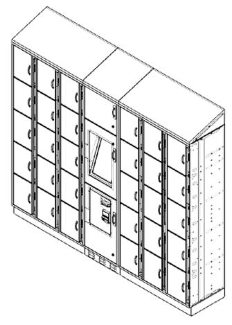
Electronic Locker System (Freedom) Electronic Locker System SS (Freedom) Internal Compartment Dimensions (7.625" W x 13.00" H x 16.875" D)
